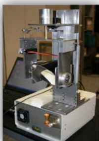
Fig. 1 Imaging system with the radiometer and the scanning antenna
