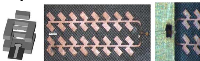
Fig. 8 From left to right - a) Waveguide-microstrip transition, b) Submillimeter wave antenna array for beam-Steering through frequency scanning, c) Array (b) with the transition (a).
